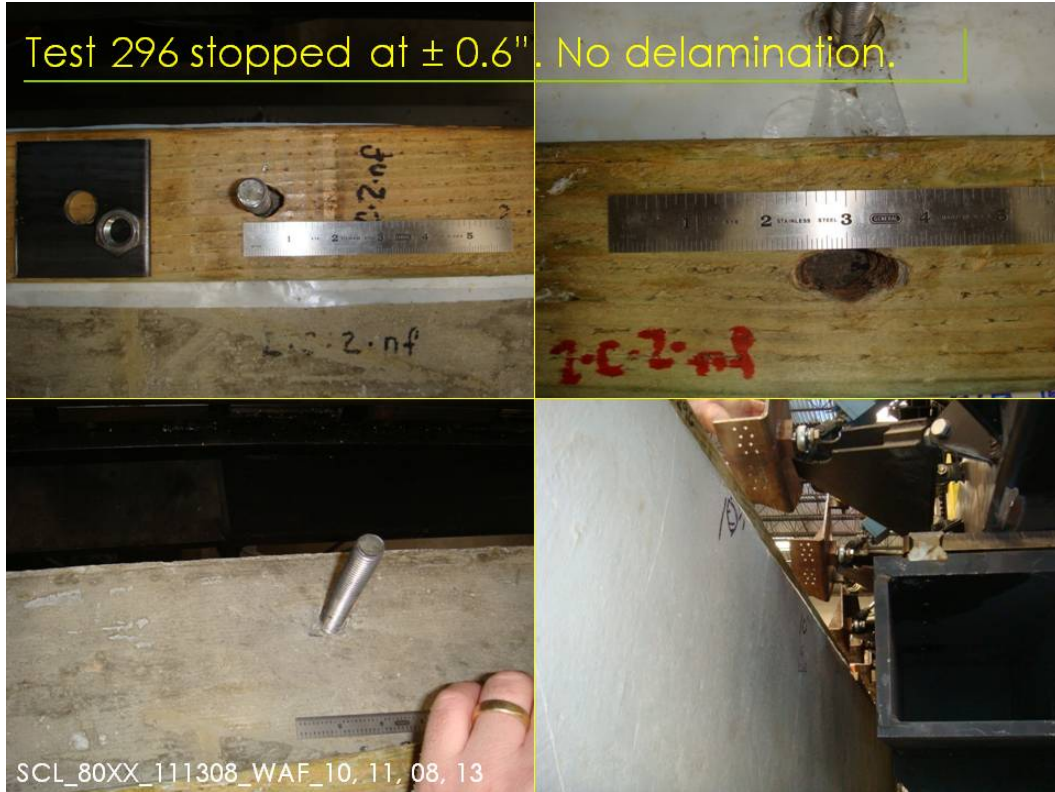
Image 6 – Composite imagery of “stopped” test (Test 296). See text for description.
