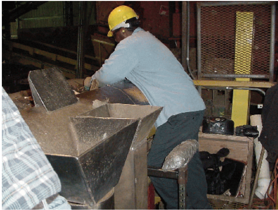
Employee standing/leaning forward to reach and sort metal materials from conveyor
