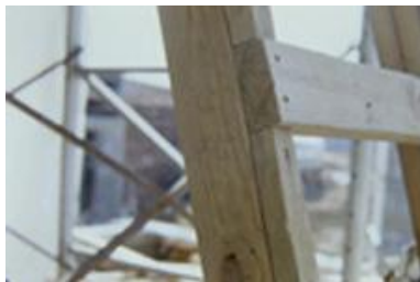
4. Job Made Ladder
