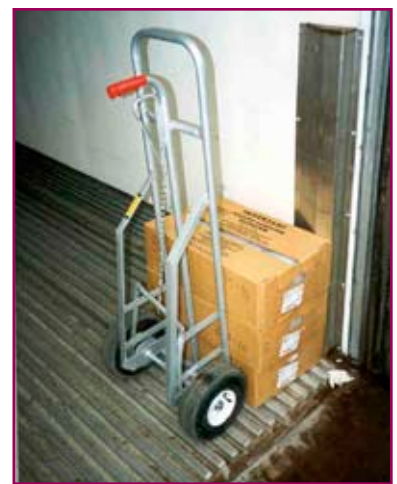
This hand truck has a brake control that slows travel on declines, reducing the physical demand for the operator.
