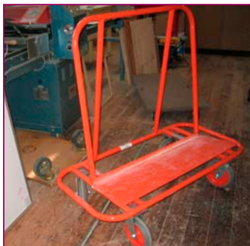
This panel cart makes carrying panel material, such as drywall, plywood, etc., an easier and safer task.
